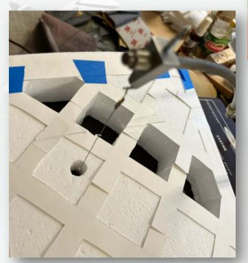
Here's a close-up of the hot wire quick disconnect on my foam cutter. The support arm is flexible and springs back up when you hook the loop
