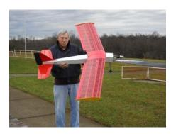
Bob Cunningham designed pattern trainer, originally for 40 size engines but converted to electric. Cunningham designed it at the behest of a man named Hooker, hence the name of the plane. The plane is receiver ready and includes a 5000mAh 4S battery, it is best described as a Stick with a swept wing. Weight is 4 pounds 10 ounces and it has a brand new Cobra motor. It is an easy plane to land and is either gentle to fly or violent if you like 3D flying depending on your setup.
